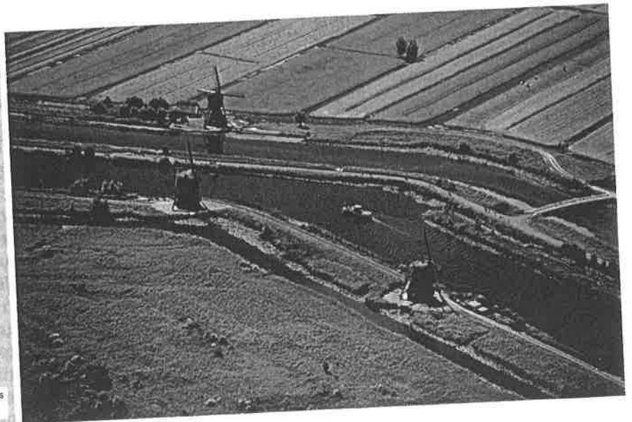
▲ FIGURE 1-44 SUSTAINABLE ECOSYSTEM: THE NETHERLANDS (left) The Dutch people have considerably altered the site of the Netherlands through creation of polders and dikes. (right) A polder in North Holland has been created by pumping the water from the site into the canal.
