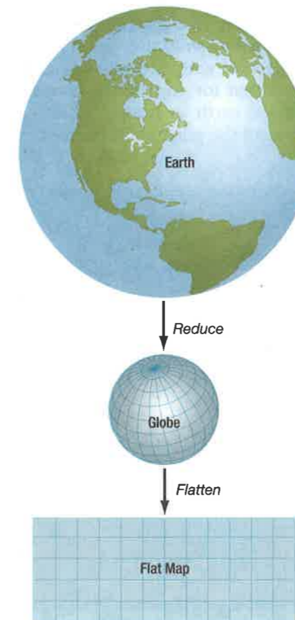
▲ FIGURE A-4 The two-step process of creating a projection.
